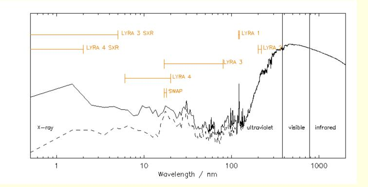
LYRA channel 1: the H I 121.6 nm Lyman-alpha line (120-123 nm) LYRA channel 2: the 200-220 nm Herzberg continuum range (now 190-222 nm) LYRA channel 3: the 17-80 nm Aluminium filter range incl the He II 30.4 nm line (+ <5nm X-ray) LYRA channel 4: the 6-20 nm Zirconium filter range with highest solar variablility (+ <2nm X-ray) SWAP: the range around 17.4 nm including coronal lines like Fe IX and Fe X
