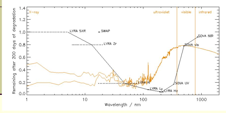
"Solar Oscillation and Variability" instrument on EURECA: **335nm, 500nm, 862nm**. (1992-1993, launched and retrieved by Shuttle) Degradation results also confirmed (?) by PICARD/PREMOS.
