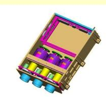
LYRA is an ultraviolet irradiance radiometer that will observe the Sun in four passbands, chosen for their relevance to solar physics, aeronomy and space weather. The instrument will detect flares and help to analyze the atmospheric composition of the Earth (Hochedez et al., 2006)
