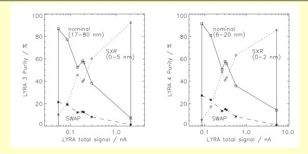
From LYRA's short-wavelength channels 3 and 4, the SWAP signal can be estimated as a subset of both the nominal signals; the SXR signals (0-5 nm and 0-2 nm) can be estimated as the complement of the nominal signals.
